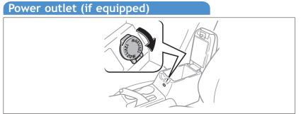
Designed for car accessories. Key must be in the "ACC" or "ON" position to use.
